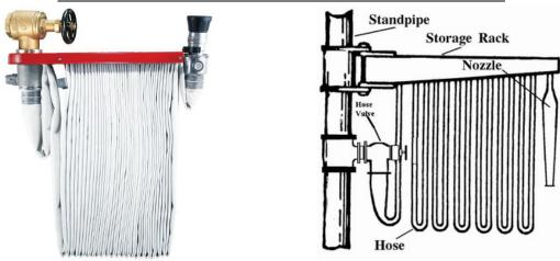
Inclined hose racks are often used, as most existing stations can accommodate such racks. The racks should be located where the sun or excessive heat will not damage the hose. The rack has the advantage of allowing the hose to drain internally while providing a drying area from which fire fighters can easily load and unload a hose.
