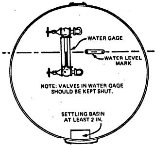
the water gauge valve, the valve shall be closed. When the valve is closed, the water and air in the tank are isolated from the sight glass. If the gauge glass breaks the volume of water and the air pressure are not affected.
