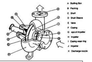
and are therefore commonly a single stage fire pumps. A typical centrifugal pump is shown in the picture below.
